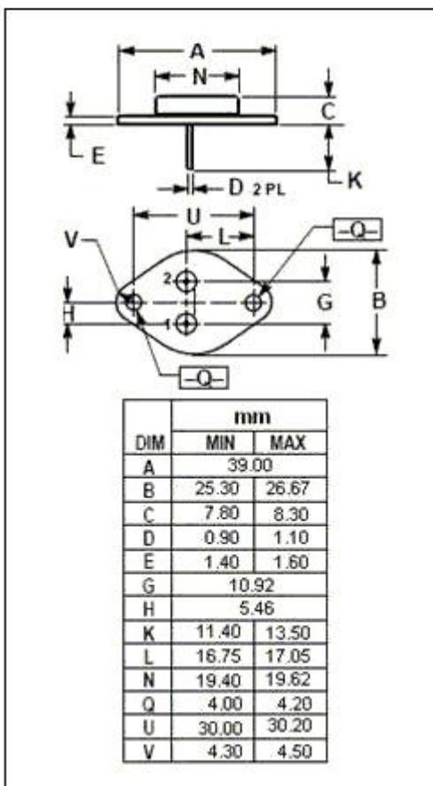
**isc Silicon PNP Power Transistor****AD149****ELECTRICAL CHARACTERISTICS**T<sub>j</sub>=25°C unless otherwise specified
